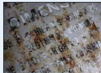
Road Salt Corrosion Damage
